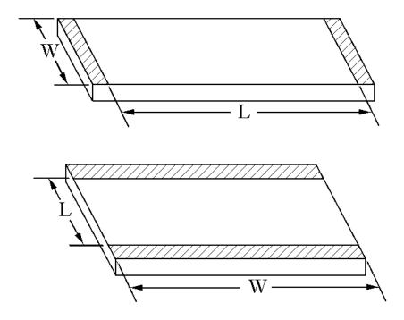
Ps = Rs x W / L = 80 ohms x W / 2 W = 80 ohms / 2 = 40 ohms.
